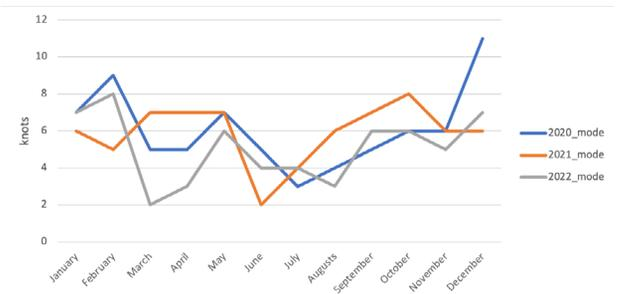
Figure 2. Wind speed – min and mode values at Lielvarde airfield from 2020 until 2022 (source: Author's developed figure)
