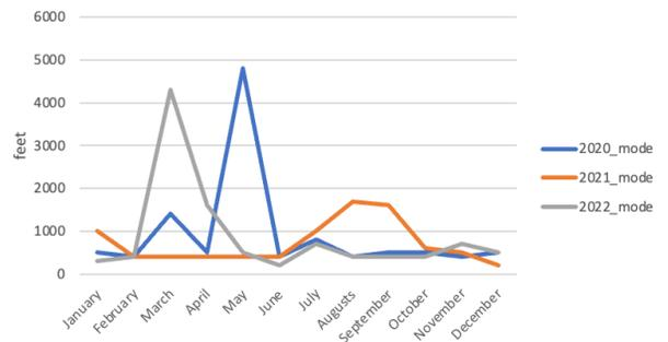
Figure 3. OVC cloud base- mode values at Lielvarde airfield from 2020 until 2022 (source: Author's developed figure)
