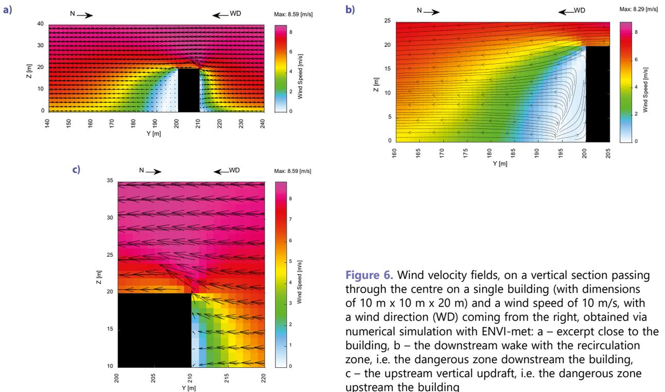
**Figure 6.** Wind velocity fields, on a vertical section passing through the centre on a single building (with dimensions of 10 m x 10 m x 20 m) and a wind speed of 10 m/s, with a wind direction (WD) coming from the right, obtained via numerical simulation with ENVI-met: a – excerpt close to the building, b – the downstream wake with the recirculation zone, i.e. the dangerous zone downstream the building, c – the upstream vertical updraft, i.e. the dangerous zone upstream the building
