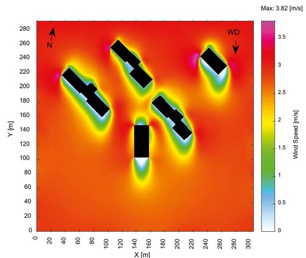
**Figure 11.** Wind velocity field in a horizontal plane close to the terrain level (9,5 m above the ground) at 12:00, extracted as an output of the ENVI-met numerical simulation of AdMaS centre with starting wind speed 4 m/s; wind comes from above
