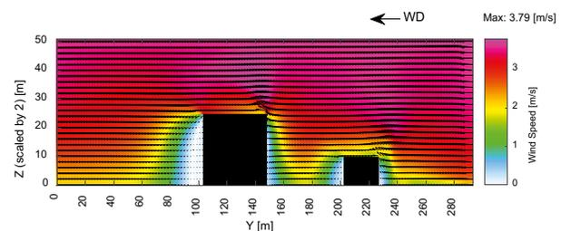
**Figure 12.** Wind velocity field in a vertical plane taken in the middle of the building H width at 12:00, extracted as an output of the ENVI-met numerical simulation of AdMaS centre with starting wind speed 4 m/s; wind comes from the right
