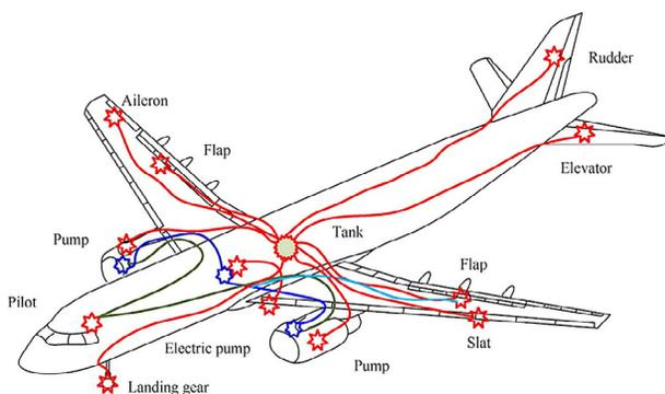
**Figure 1.** Distribution of aircraft hydraulic pipeline system (Gao et al., 2021)
