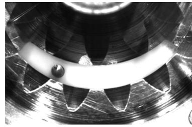
**Figure 4.** View of the insert made of POM – without modification,  $n = 1000$  rpm (source: own work)
