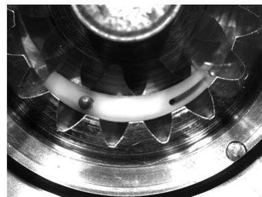
**Figure 6.** View of the modified insert made of PA – first modification,  $n = 1000$  rpm (source: Towarnicki et al., 2023)
