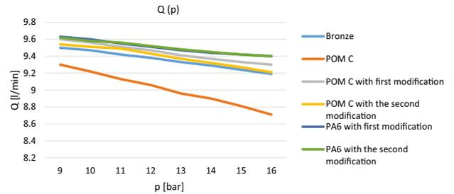
**Figure 10.** Characteristics of the change in pump performance depending on the change in pump discharge pressure for various materials and with type I and II modifications,  $n = 1000$  rpm
