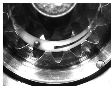
**Figure 8.** View of the modified insert made of PA – second modification,  $n = 1000$  rpm (source: Towarnicki et al., 2019)
