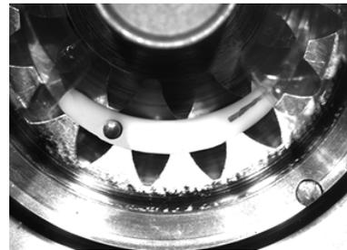
**Figure 5.** View of the modified insert made of POM – first modification,  $n = 1000$  rpm (source: Towarnicki et al., 2023)
