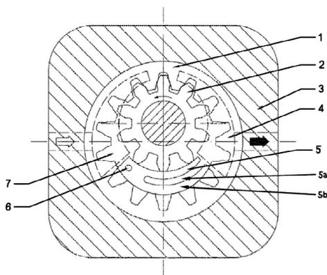
**Figure 2.** Cross-section of the pump with a modified sickle insert: 1 – toothed rim, 2 – gear wheel, 3 – pump body, 4 – discharge space, 5 – sickle insert, 5a – bay inside the sickle insert, 5b – elastic tongue of the sickle insert, 6 – locating pin, 7 – suction space (Towarnicki et al., 2021)
