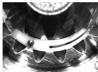
**Figure 7.** View of the modified insert made of POM – second modification,  $n = 1000$  rpm (source: Towarnicki et al., 2023)
