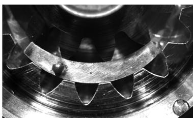
**Figure 3.** View of the insert made of bronze B101 – without modification,  $n = 1000$  rpm (source: own work)
