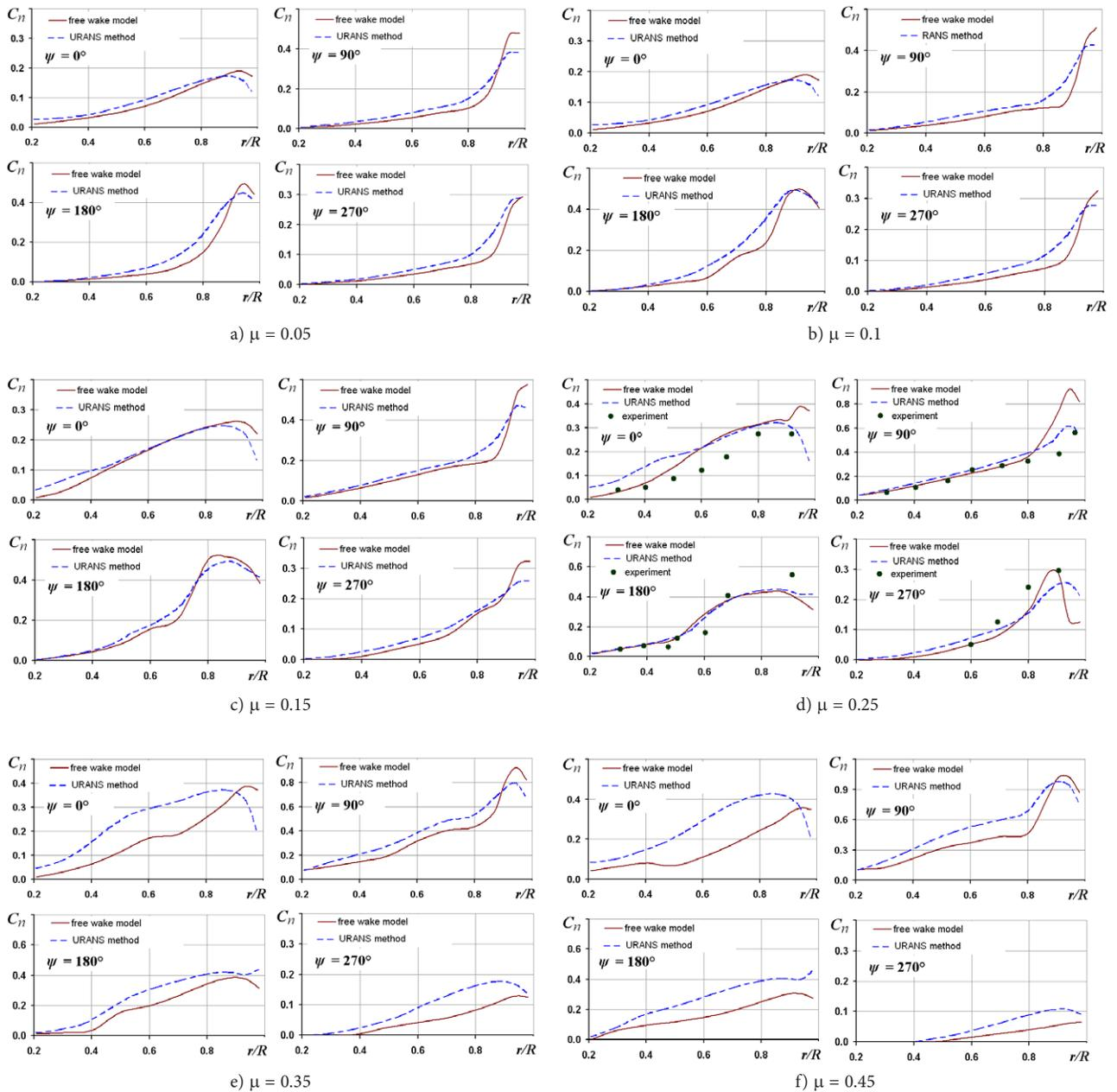
Figure 6. Comparison of normal force coefficient distribution  $C_n = f(r/R)$  at various blade azimuthally location by URANS method and free wake model
