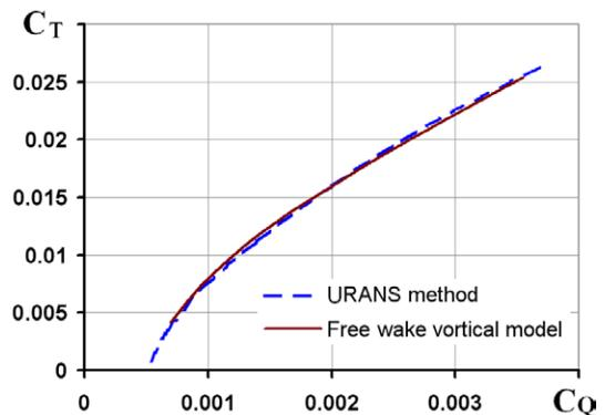
Figure 4. Calculated dependences of  $C_T = f(C_Q)$  in hover
